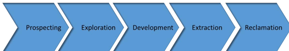
Figure 2: Phases of the mining process.
