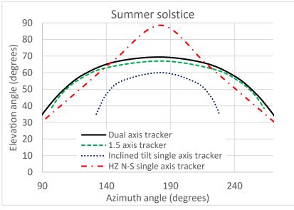
Figure 1: Trajectories of different types of solar trackers
