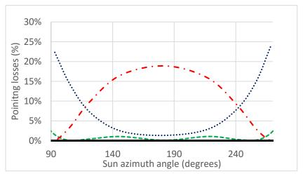
Figure 2: Pointing losses of different tracking systems
