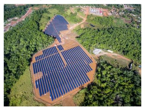
Voltalia added a 4 MW solar power plant to diesel gensets in Oiapoque in Brazil (source: Voltalia)
